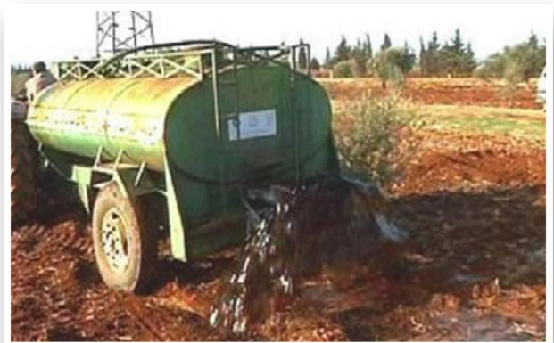
Figure 2: OVW spreading between the olive orchard rows
